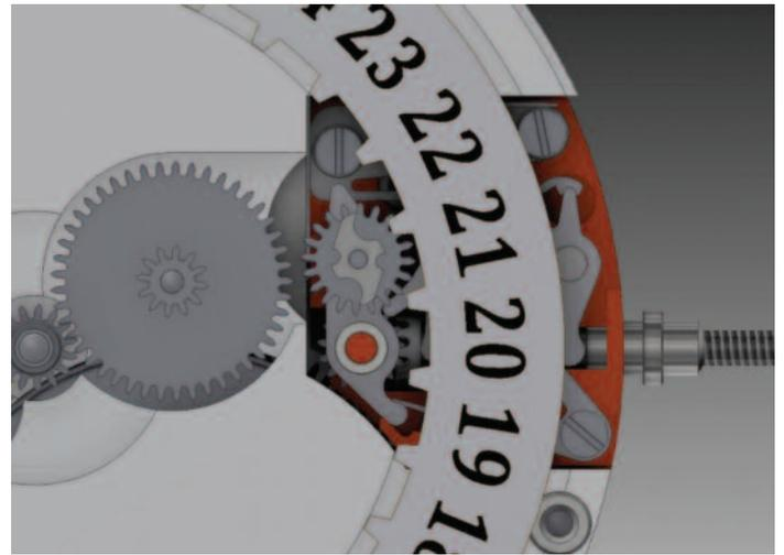
The quick-set mechanism with the date ring in place.
